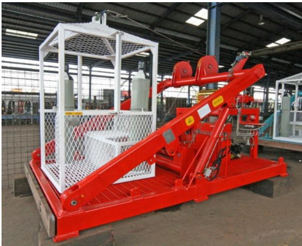
1 x Diver LARS – The Launch And Recovery System comes complete with a 2- diver dive basket c/w air cylinders, 2 x man-riding certified winches (1 x hydraulic winch & 1 x clump winch), 200kg clump weight, built in hydraulic power pack, hydraulic 3-bank spool valve, rams and on-board controls.
