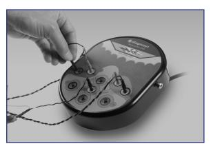
32-Bit Amplifier Unprecedented 1 nano Volt resolution and illuminated receptacles guide lead insertion and eletrode contact quality
