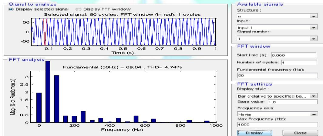
Figure 8. FFT analysis of current waveform with filter
