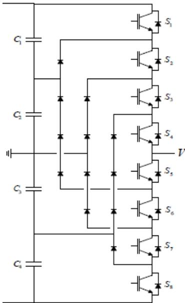
Figure 1. Diode clamped multilevel
