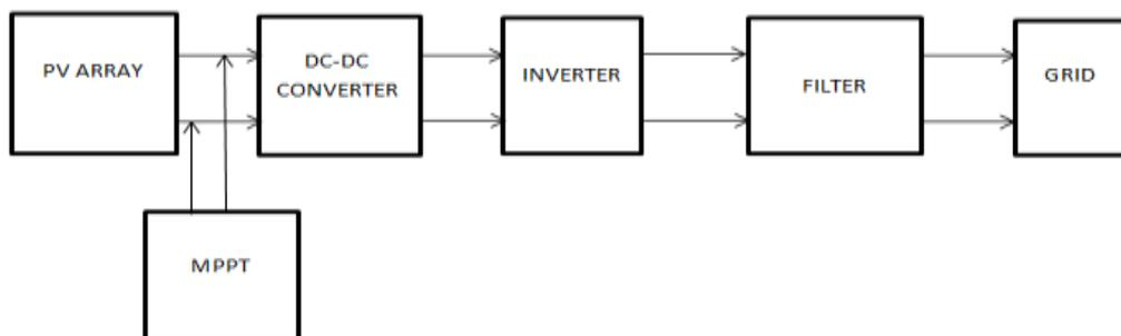
Figure 4. Block diagram of grid connected PV system
