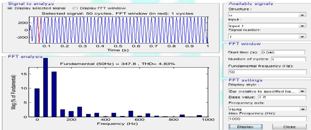
Figure 7. FFT analysis of voltage waveform with filter
