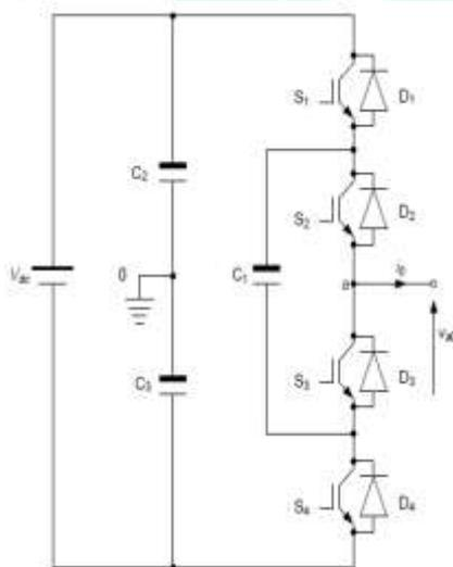
Figure 2. Flying capacitor multilevel inverter
