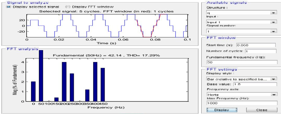
Figure 6. FFT analysis of the current waveform without filter
