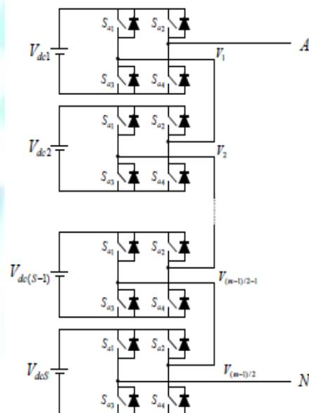
Figure 3. Cascaded multilevel inverter
