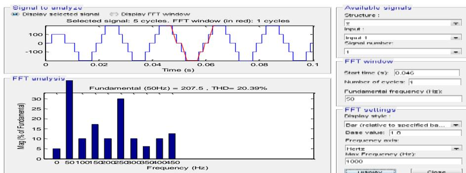
Figure 5. FFT analysis of the voltage waveform without filter
