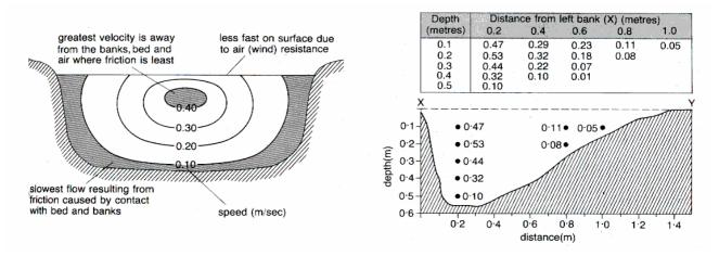
In the Lyn, velocity increases with distance from the source but there are considerable small-scale local variation, particularly between pools and riffles and with distance from the bed and banks. Velocity is also influenced by the bed roughness which also creates turbulence in the flow.
