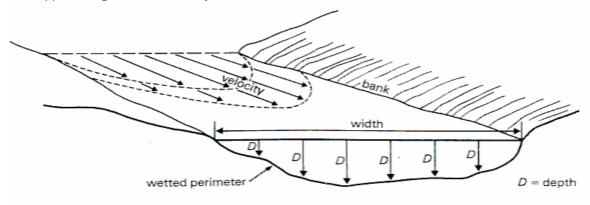
Efficiency (Hydraulic radius). Channel efficiency can be measured by the hydraulic radius which is ratio between the cross sectional area and the wetted perimeter. The wetted perimeter is the length of the bed and banks in contact with the water. (This will vary with the rate of discharge).
