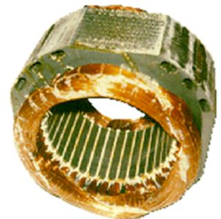
**Figure 2: A motor stator with pinhole insulation damage.**
