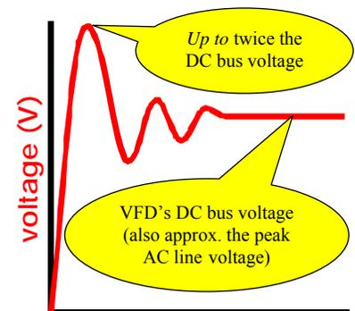
Figure 6: Voltage levels in a PWM pulse.
