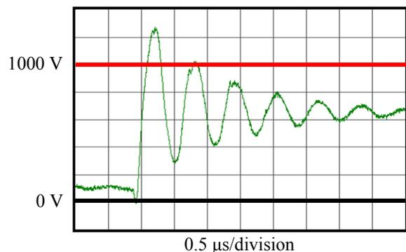
**Figure 7: A PWM Pulse with a high  $dV/dt$  value can cause a large voltage overshoot.**
