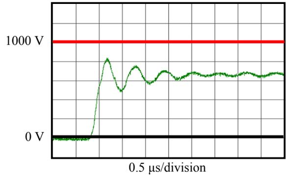
Figure 8: A PWM pulse with a lower  $dV/dt$  value creates a lower voltage overshoot.
