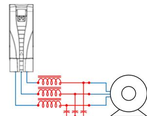
Figure 12: A  $dV/dt$  filter reduces the rate of rise of the PWM pulse and controls voltage overshoot.
