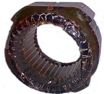
Figure 1: A motor stator with over-heated insulation.
