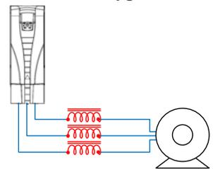
Figure 11: A set of output reactors between the VFD and the motor.
