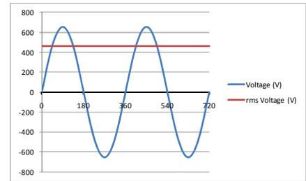
Figure 5: The relationship between instantaneous and rms AC voltage.
