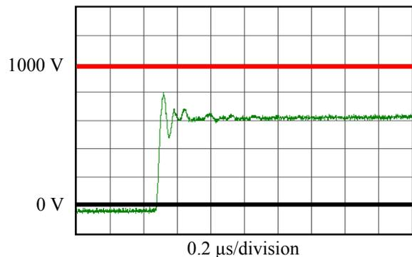
Figure 9: A short motor cable length causes a low peak voltage.
