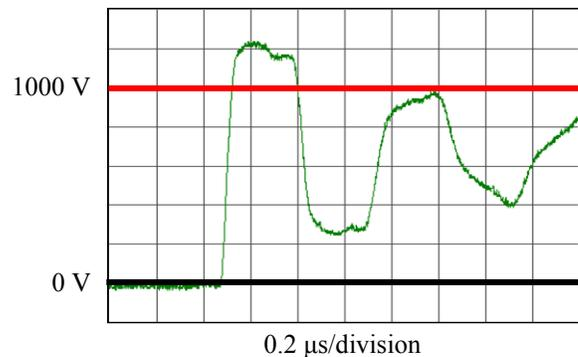
Figure 10: A motor cable length over 200 feet causes a large voltage overshoot.
