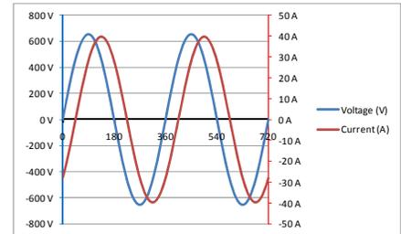
Figure 3: In an AC induction motor, current lags behind voltage.
