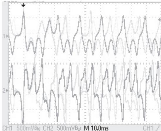
Fig. 5:  $V_x(t)$  and  $V_y(t)$  waveforms from a Lorenz attractor
