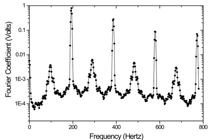
Fig. 8: Spectrum of attractor in a ‘periodic window’ – note the onset of a sub-harmonic spectral line
