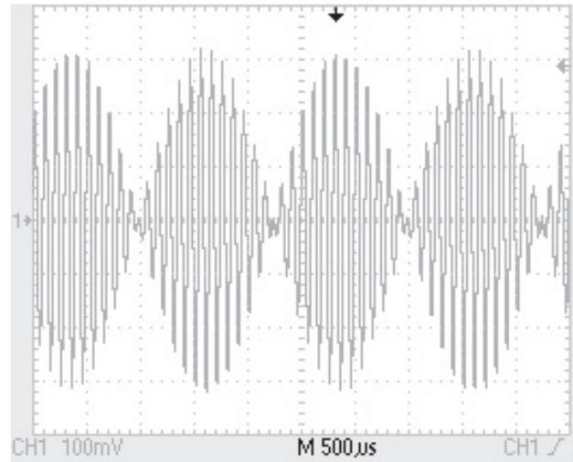
Fig. 3: The waveform of a simple product of two sinusoids
