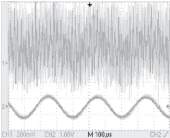
**Fig. 9: 3.3-kHz sinusoidal signal, corrupted by interference**
