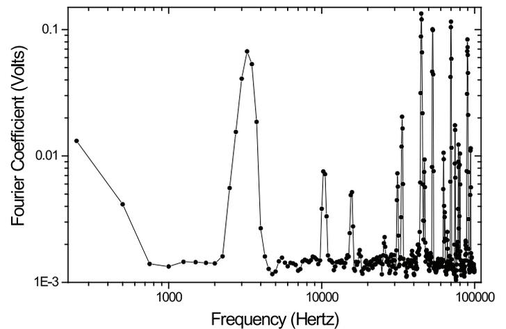
**Fig. 10: The Fourier spectrum of a 3.3-kHz signal and the interference at 45-kHz (and harmonic)**
