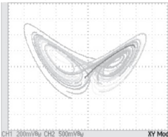
Fig. 6:  $V_z$  (up) and  $V_x$  (across) in a parametric plot of chaos
