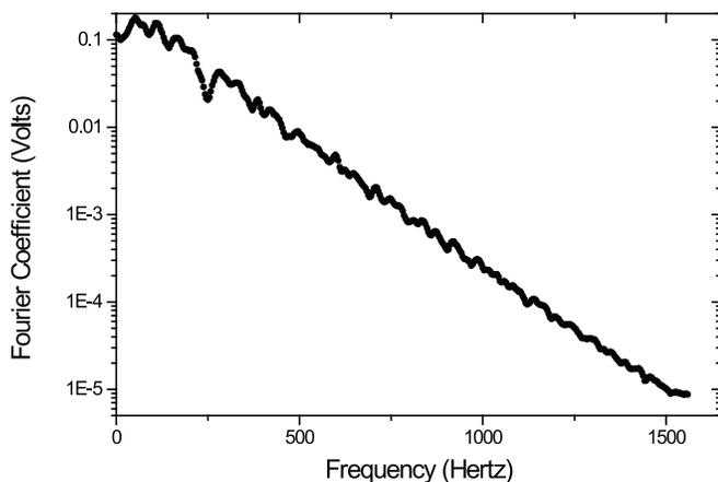
Fig. 7: The Fourier spectrum of Fig. 5’s chaotic waveform
