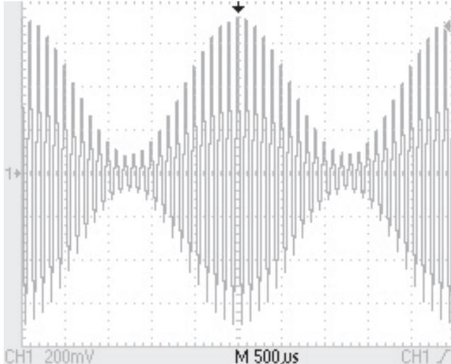
Fig. 1: An amplitude-modulated 10-kHz waveform
