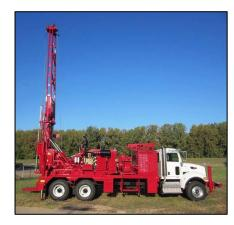
Most well drilling rigs are over the legal road limit for both gross and axle weights, based on their configurations. This is due to the
