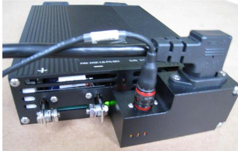
The supply is designed to be used with the voltage sense feature. Voltage sense is automatically activated when an appropriate loom is plugged into the sense connector. When there is no connection to the sense connector of the power supply it will be disabled and there will be no voltage output. To use the supply without voltage sense, a blanking plug must be used on the sense connector. See connector interface section for details.
