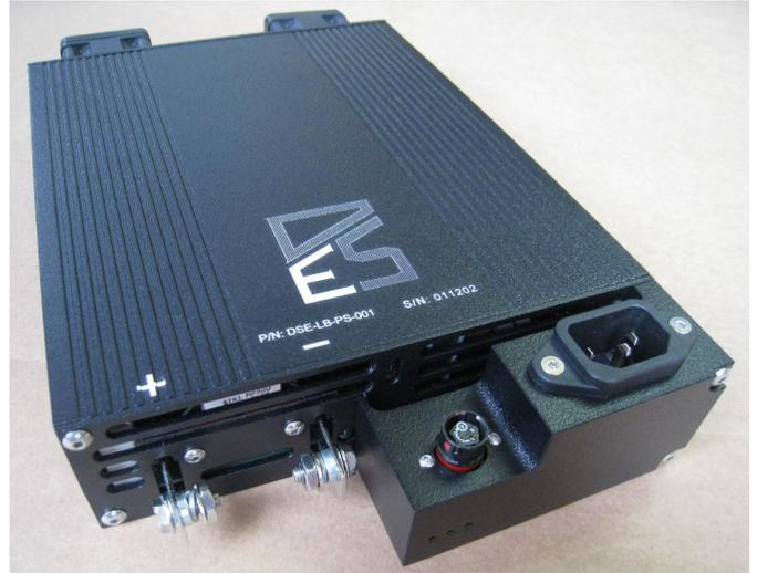
Three LEDs on the front of the enclosure indicate (from left to right) Power On, Voltage Sense Enabled, and Voltage within the acceptable tolerance. Under normal operation all 3 LEDs should be illuminated. With a blanking plug (operation without voltage sense), the center LED will not be on.
