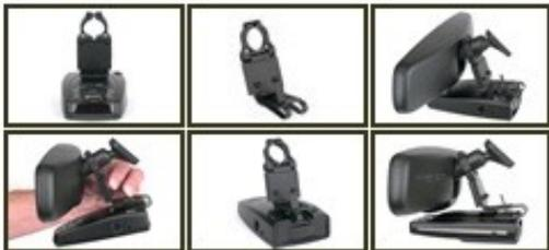
BlendMount BBE-2000 radar mount, used a BlendMount mirror tap (to tap into the power in the rear view mirror) to power the camera, and mounted the camera to the radar mount using a mini ball head camera mount. It turned out to be a nice install ... no wires visible and when driving, the camera is hidden by the rear view mirror, so no obstructed view.
