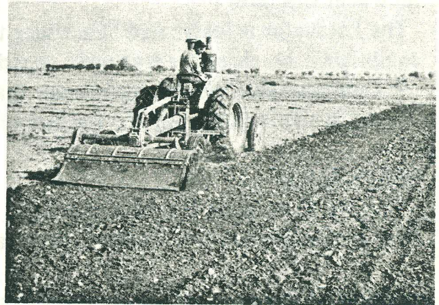
Tilth control demonstrated—by using the shield. Greater variation still can be obtained with 'Selectatilt'. ('H' trailing Rotavator on the same field—West Pakistan).
