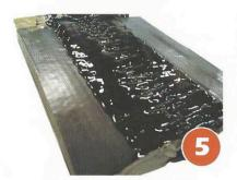
Once the splice is fully sealed, or the fastener is fully covered, leave to cure for the following times before commencing belt operation:
