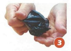
Mix by kneading and squashing the resin pack together until it starts to warm up (2-3 minutes).
