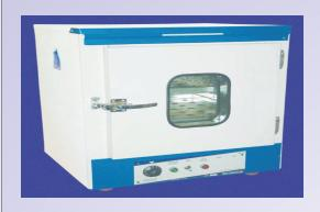
Double walled inside made of thick Aluminum or S.S. outer made of M.S. duly finished with enamel paint. Thermostatically/ Digital controlled. Temp. 5°C above room temp. to 65°C Accuracy  $\pm$  1°C . Door has double viewing window to observe the sample placed inside the chamber without disturbing the thermal condition. Complete with accessories.
