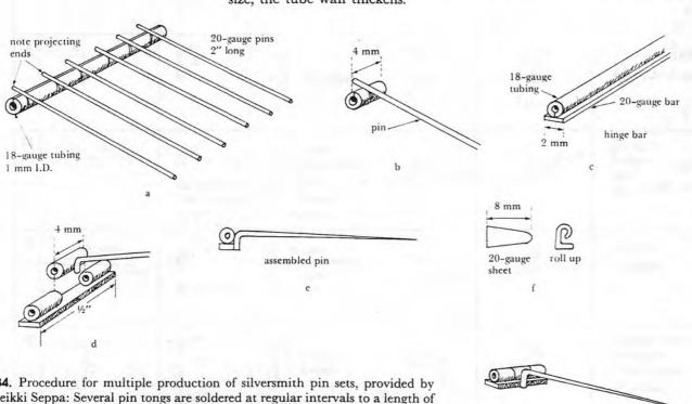
434. Procedure for multiple production of silversmith pin sets, provided by Heikki Seppa: Several pin tongs are soldered at regular intervals to a length of tubing (a), which is then cut apart (b). A length of identical tubing is soldered to a bar (c) and cut to form a three-section hinge with the pin (d), whose projecting end is bent down to provide spring tension against the bar (e). Finally, a simple clasp is rolled from sheet (f) and positioned on the work to receive the pin tong (g).
