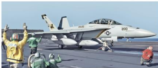
The AN/ASD-12 Shared Reconnaissance Pod (SHARP) was used on F/A-18Fs for several years to provide the carrier air wing with a tactical reconnaissance capability. Here, the CAG Super Hornet assigned to the "Blacklions" of VFA-213 is prepared for launch from USS THEODORE ROOSEVELT, CVN-71. It has a SHARP pod loaded on the centerline station, but it is also armed with 500-pound GBU-38(V)2 JDAMs for the mission. (U. S. Navy)
