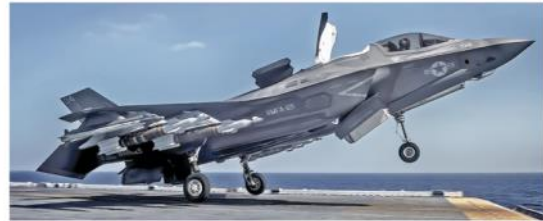
Above: When stealth is not a mission requirement, ordnance can be carried externally on six pylons under the wings. Here, an F-35B assigned to VMFA-211 takes off from USS WASP, LHD-1, with laser-guided bombs on its inboard and mid-wing pylons, and an AIM-9X Sidewinder is on the outboard wing station. Note that the F-35B has a single wheel on the nose gear. (U. S. Navy)
