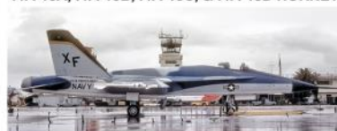
The second of the two YF-17s was acquired by the Navy for use as a developmental aircraft for the F/A-18 Hornet, is shown here in a blue and grey camouflage scheme and Navy markings in December 1978. F/A-18 PROTOTYPE
