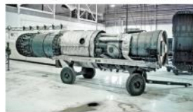
The Pratt and Whitney J75-P-8 engine was chosen to power the Crusader II. This powerful engine could develop 18,500 pounds of thrust in military power and 26,000 pounds of thrust in afterburner. Different versions of the J75 powered several military and commercial aircraft, most notably the F-105 Thunderchief and the F-106 Delta Dart. (Continued)
