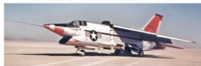
The first of the three flying XF8U-3 Crusader II prototypes, BuNo. 146346, poses on the dry lakebed at Edwards Air Force Base, California. Like the standard Crusaders, the Crusader II featured a variable incidence wing and full span leading edge droops. Both features are visible in this view. Three radar-guided Sparrow missiles were carried semi-recessed under the forward fuselage. (NMAA)
