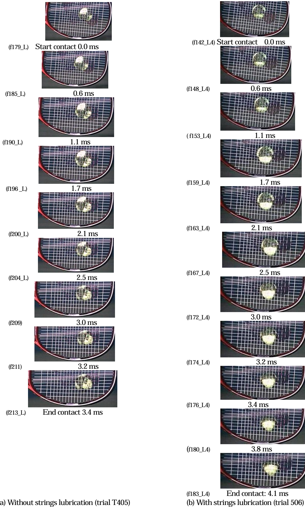
Fig.6 Effect of lubrication of used strings on the ball spin behaviors (impact views from back side direction with frames per 10^{-4} s). (a) Without lubrication (b) With lubrication of used strings
