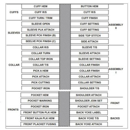
Figure 5 - Progressive Bundle system for shirt making
