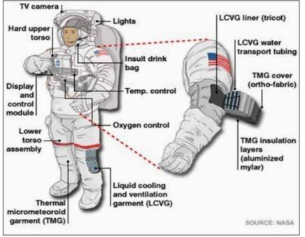
Figure 1 - Different parts of a space suit (EMU)
