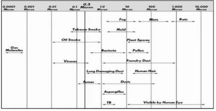
Fig. 2: Comparative size chart of different particulate matters in the air
