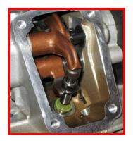
Use the included feeler gauge to measure the opening gap: the gap between the opening rocker arm and the opening shim. Begin measuring
