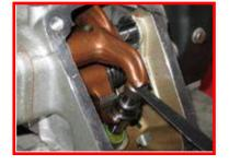
Record the measurement on the accompanying worksheet. Record this as measurement: **A**. Record the Ducati recommended clearance in column **B**. Compare the two measurements. If **A** is greater than **B** (if the measured is greater than the recommended), subtract and record the result in column **C**.
