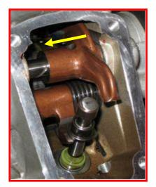
Put Opening shim onto valve stem
