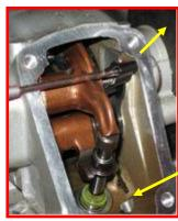
If either the opening or the closing shims require replacement to bring the gap(s) into specification follow this procedure.
