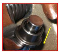
Obtain the correct shim(s) and reassemble the valve train. Slide the closing shim onto the valve stem, narrow side slides onto the valve stem first.
