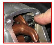
Once the valve is reassembled, re-check the clearances to verify the valve train is within specification. With the cam belts installed, rotate the engine to verify smooth operation. Reassemble as required.
