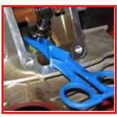
Press down on the Closing rocker to expose the retaining rings. Slight engine rotation may be required to get the rocker to move far enough to expose the retaining rings. The retaining rings are in two halves.
