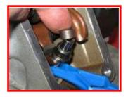
Remove the Opening shim from the valve stem.
