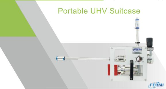
This is an easy to transport UHV Suitcase, it is leak tested and baked out to UHV standard before shipment, thus it is ready to use at the time of open box. There is a combination pump (lon/ NEG) keeps the inner volume constantly in UHV environment even at the shortage of power, thus it is an ideal tool for carrying sensitive samples for remote instruments.
