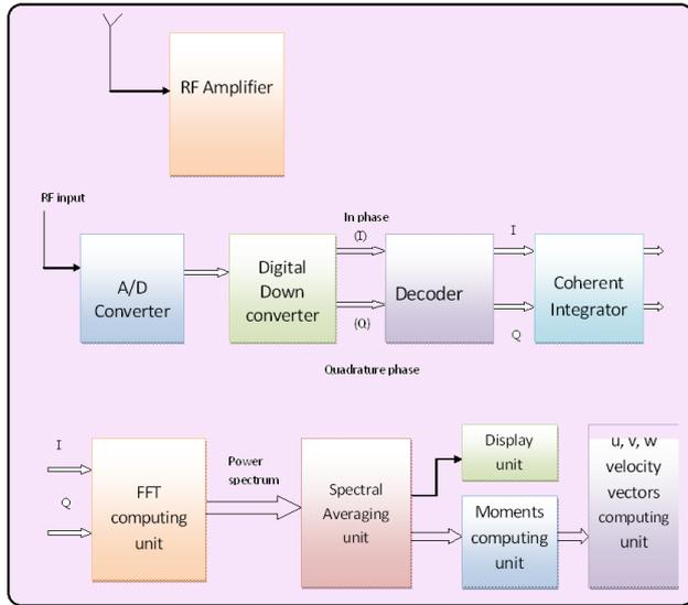
Figure 3 Subunits of the Data Acquisition system
