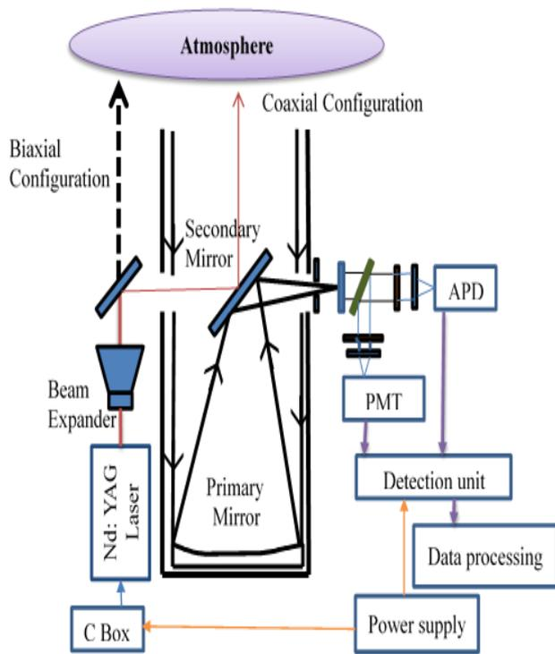
Figure 4. Schematic diagram of the lidar system developed
