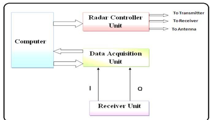
Figure 1. Block diagram of Data Acquisition and a processing unit for Atmospheric Radars
