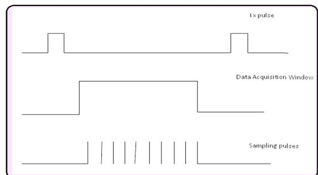
Figure 2. A timing diagram for Data Acquisition
