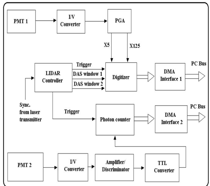
Figure 11 Block diagram of data acquisition system
