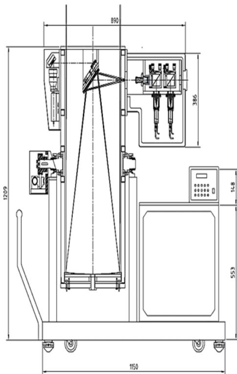
Figure 5. Mechanical drawing of the Lidar system
