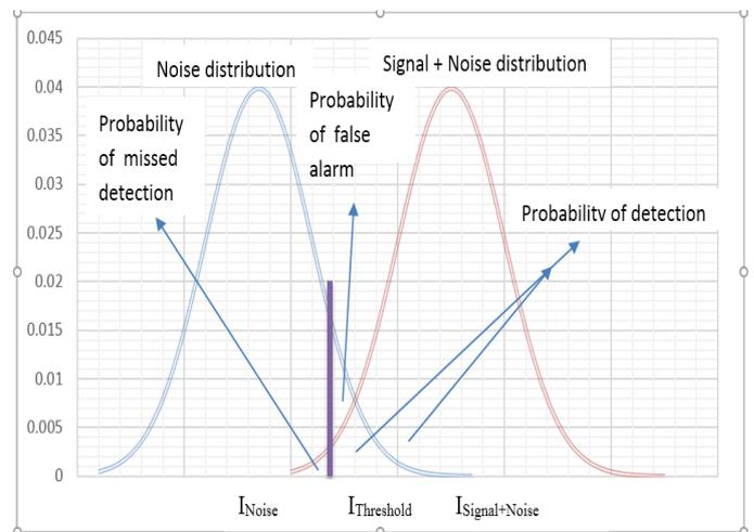
Figure 7 PDF of a Lidar return
