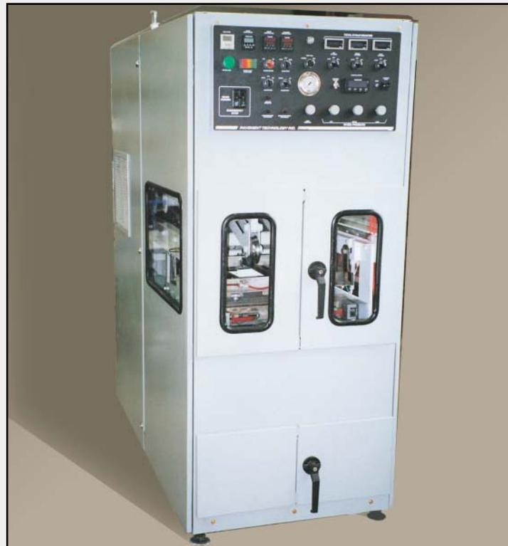
*Many DOTs, producers, and researchers use performance testing as a way to prove the viability of asphalt mixes prior to construction. The Asphalt Pavement Analyzer is the equipment of choice for much of that testing.*
