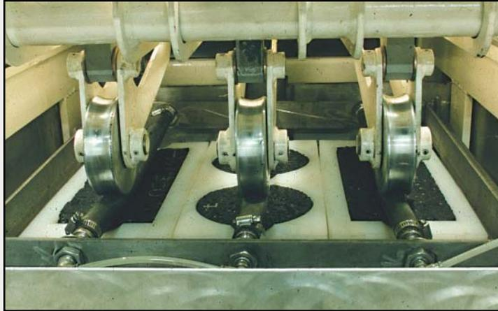
The Asphalt Pavement Analyzer (above) from Pavement Technology, Inc. is capable of conducting a range of performance tests, including the rut test on three material samples that is shown in this photograph. An example of one of the APA’s tests is shown in the graph (below) that illustrates the relationship between binder content and APA rut depth for mix-design purposes.
