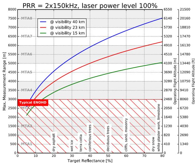
**Example:** VQ-1560 II at 2 x 150,000 pulses/sec, laser power level 100%
