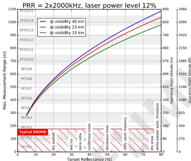
**Example:** VQ-1560 II at 2 x 2,000,000 pulses/sec, laser power level 12%
