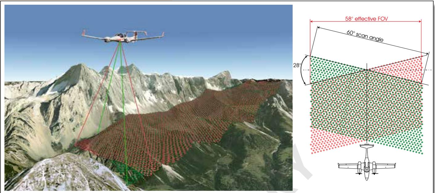
Each channel delivers straight parallel scan lines. The scan lines of the two channels are tilted against each other by 28 degrees providing an optimum distribution of the measurements on the ground invariant to changes in terrain height.
