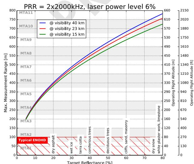
**Example:** VQ-1560 II at 2 x 2,000,000 pulses/sec, laser power level 6%
