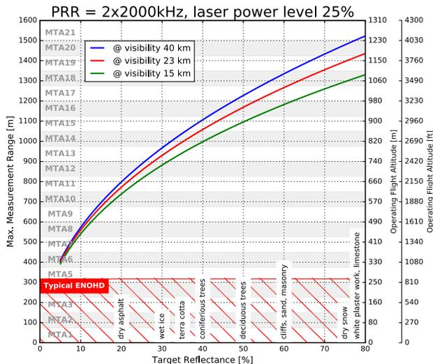
**Example:** VQ-1560 II at 2 x 2,000,000 pulses/sec, laser power level 25%
