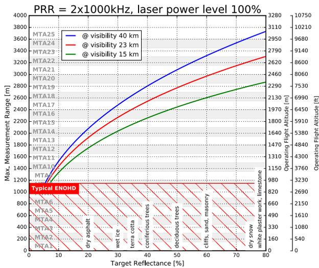
**Example:** VQ-1560 II at 2 x 1,000,000 pulses/sec, laser power level 100%
