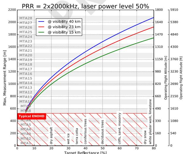
**Example:** VQ-1560 II at 2 x 2,000,000 pulses/sec, laser power level 50%
