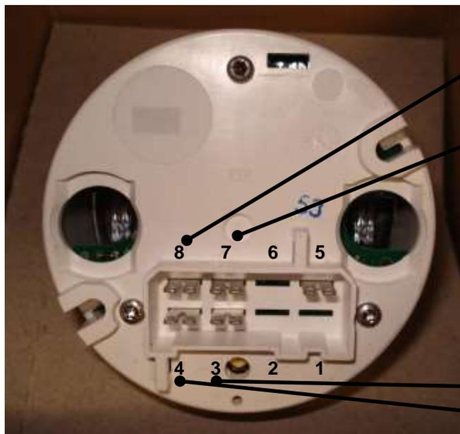
Connect to Red Wire of tachometer pick-up
