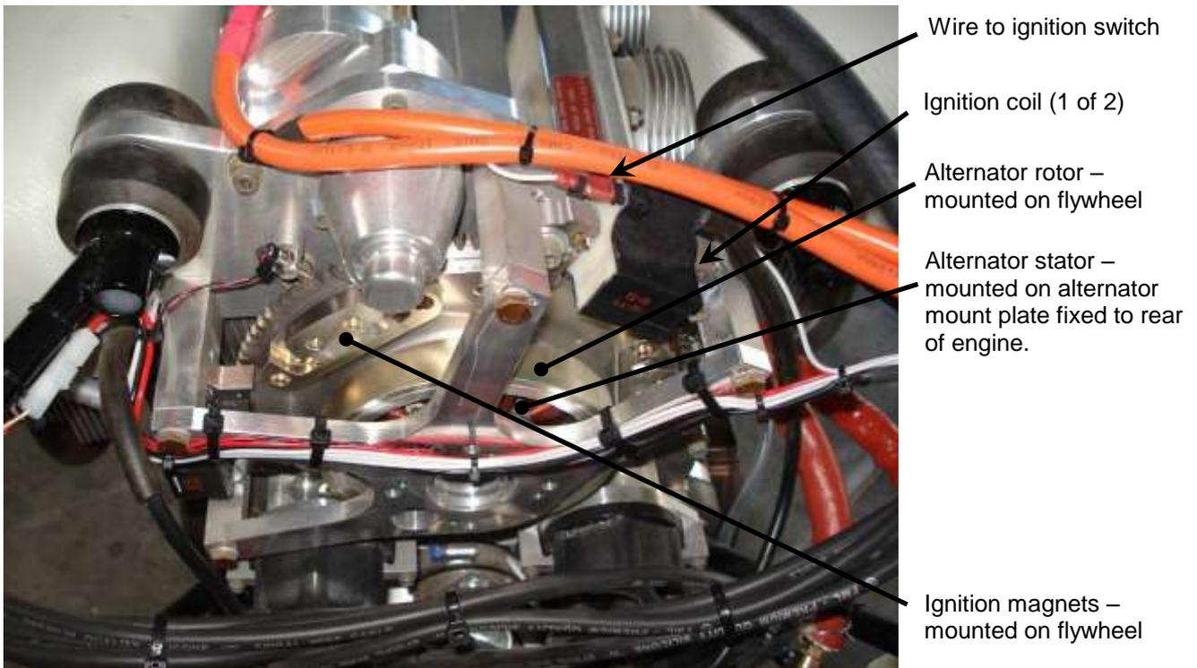
Figure 9. Ignition & Alternator Detail
