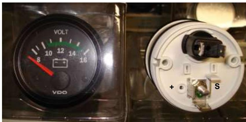
Figure 21. Voltage Gauge Connections
