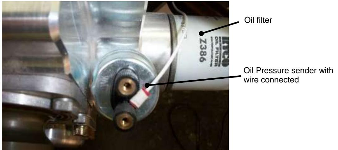
Figure 19. Oil Pressure Sender
