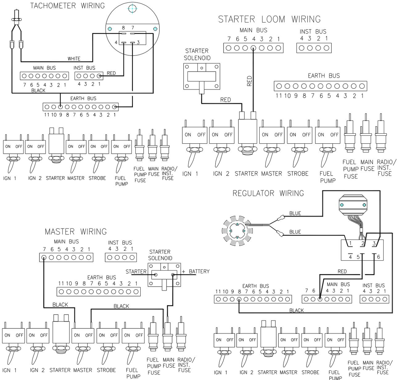
Figure 63. Wiring Details
