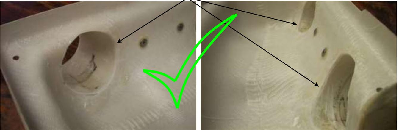
**Figure 35. Air Filter Box Plumbing – Correct**
