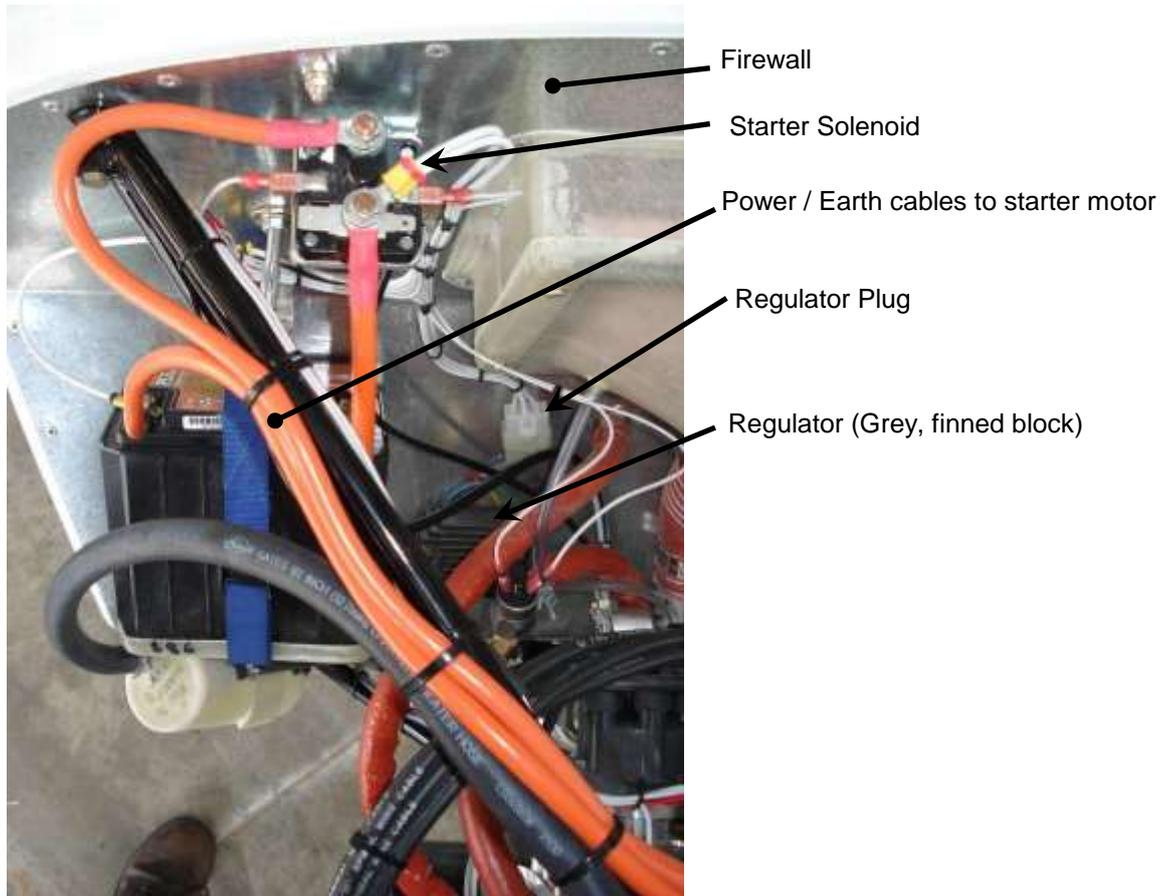
Figure 11. Electrics Installation to Firewall
