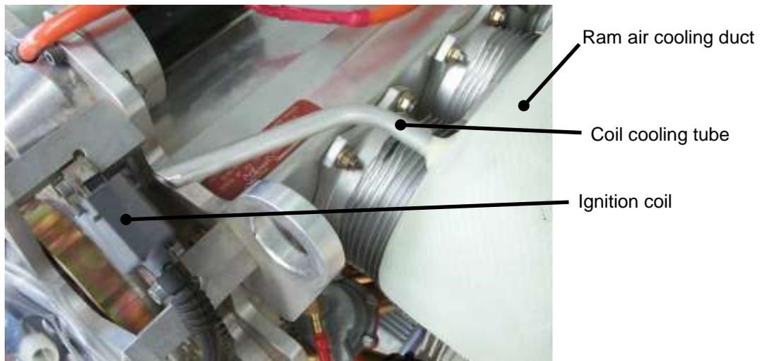
Figure 13. Ignition Coil Cooling Tube
