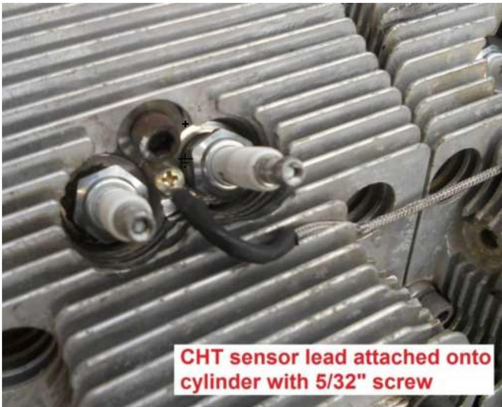
Figure 24. CHT sensor between plugs
