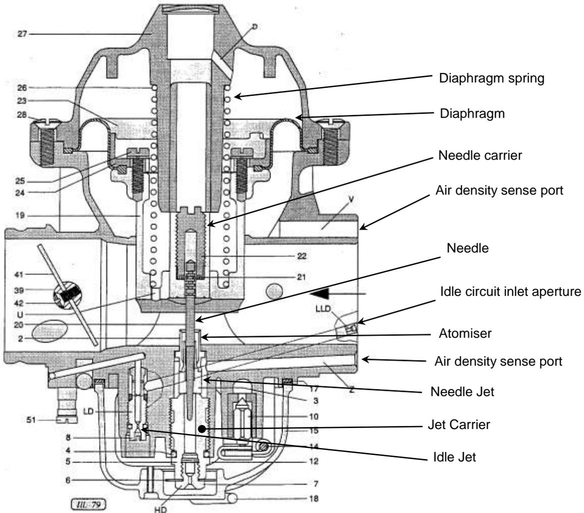
Figure 31. Carburettor Schematic
