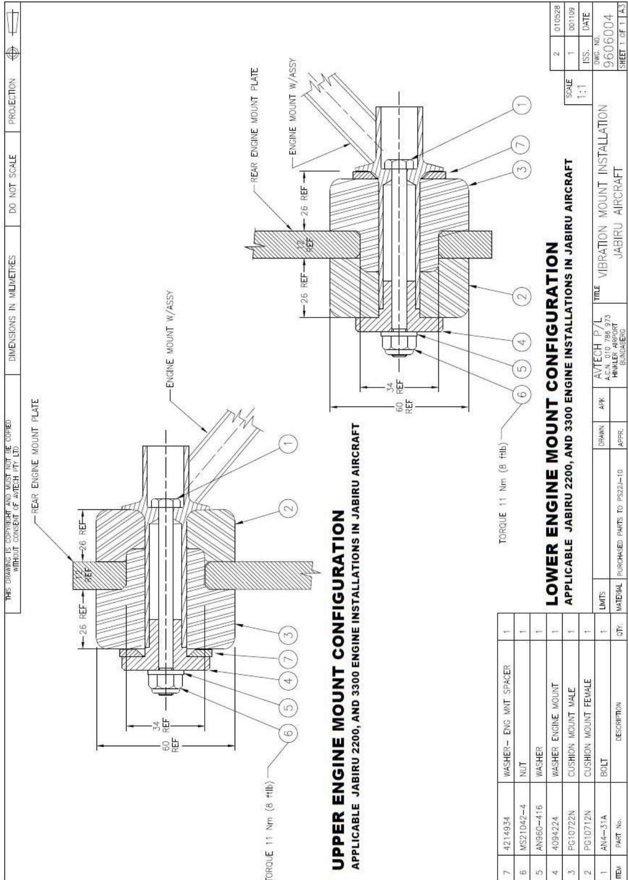
Figure 42. Engine Mount Detail
