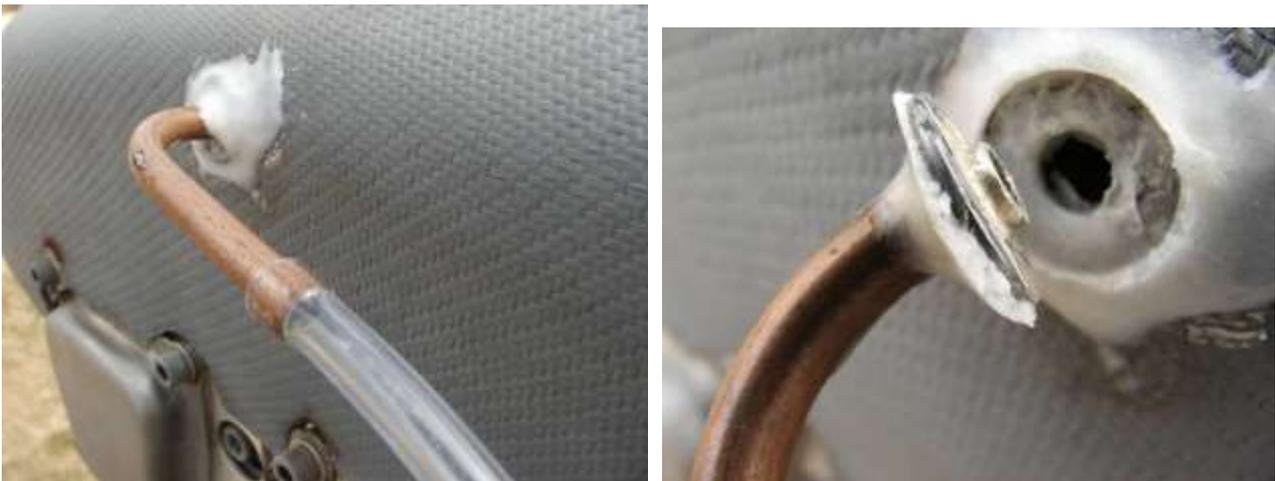
Figure 61: Ram Air duct pressure tapping.
