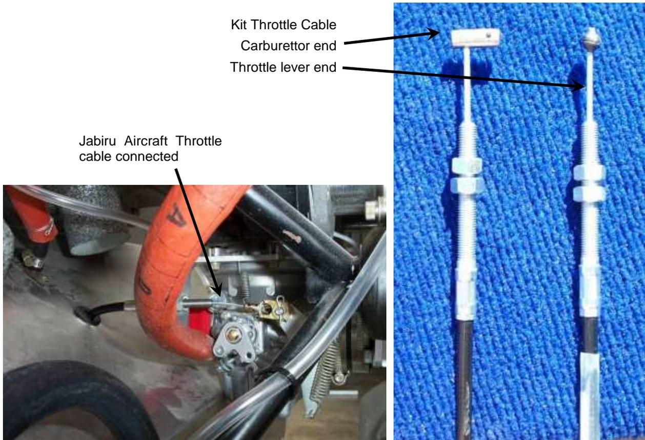
Figure 46. Control Connections to Carburettor
