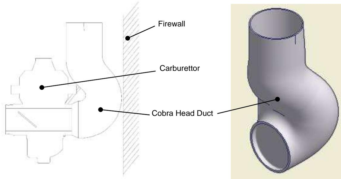
Figure 37. Cobra Head for Installations with Minimum Carburettor Clearance
