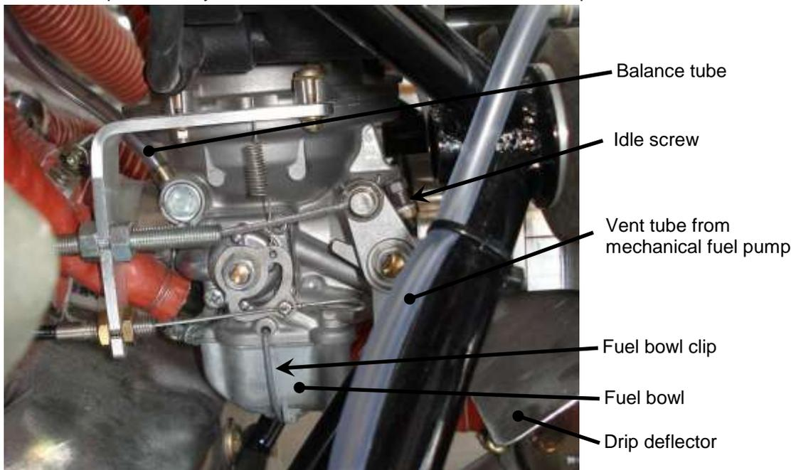
**Figure 29. Carburettor Installation**
