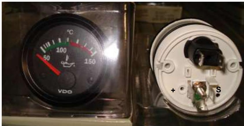
Figure 18. Oil Temperature Connections
