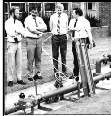
Picture 2. Performance testing of deluge valve assembly at Wormald Fire Systems, Ashfield NSW. From left to right: Peter Setright, Bill Fleming - Transfield Kumagai, Berndan White - Roads and Traffic Authority and Rick Foster - Eagle Consulting Group.
