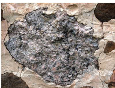
Granite with large enough crystals to be called pegmatite. Pink crystals are potassium feldspar, black minerals are dominantly biotite, and gray is predominantly quartz.
