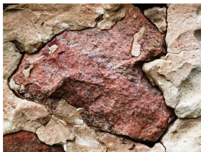
This is granite – it resembles granite from the Montello batholith, which is characterized by a red (or pink) color and paucity of ferromagnesian minerals. This is an example of the Wisconsin state stone, which is red granite.
