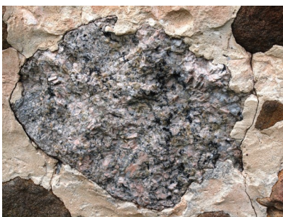
Granite with large enough crystals to be called pegmatites. Large crystals are feldspar, biotite, and quartz. Biotite is also predominant.
