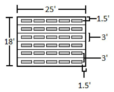
If designed as a conventional trench formation, the resulting footprint would be approximately  $1,500 \text{ ft}^2$ . The above PPBPS bed formation offers a 70% reduction in area needed on the lot.
