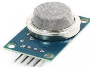
The MQ 135 Quality Detector Sensor Module For Arduino has lower conductivity. When the target combustible gas exists, the conductivity of the sensor is higher along with the gas concentration rising. The MQ 135 sensor has high sensitivity to Ammonia, Sulphide and Benzene steam, also sensitive to smoke and other harmful gases
