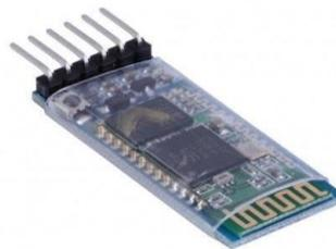
Bluetooth is a wireless technology standard for exchanging data over short distances using short-wavelength UHF radio waves in the ISM from 2.4 to 2.485 GHz from fixed and mobile devices, and building personal area networks. The first channel starts at 2402 MHz and continues up to 2480MHz in 1MHz steps. It usually performs 1600 hops per second, with Adaptive Frequency-Hopping (AFH) enabled.
