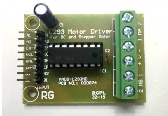
Motor driver is a double H bridge drive chip - L293DN with voltage range of 5V-12V and current range of 0-36mA. Maximum power consumption is 25W, dimensions: 43 x 43 x 26mm, weight: 26g and a built-in 5v power supply, when the driving voltage is 7v-12v.
