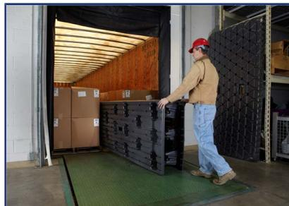
After learning about Paylode's resilient polyethylene Bulkhead Spacers, Lyons Magnus conducted test shipments from Fresno, Calif., to its sister plant in Kentucky. The company concluded the lightweight interlocking void fillers were much easier to handle and load. Furthermore their ability to absorb energy without crushing-up to 20,000 lbs. of force-meant that the spacers could be reused for well over one hundred turns.
