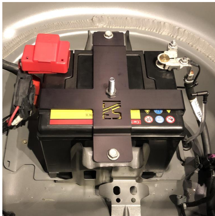
Battery kit installed in a 2015 Camaro Z/28
