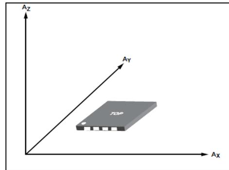
Fig 3: "ADXL335 three axis measurement"
