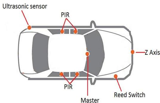
Fig 1: Vehicle with sensor network
