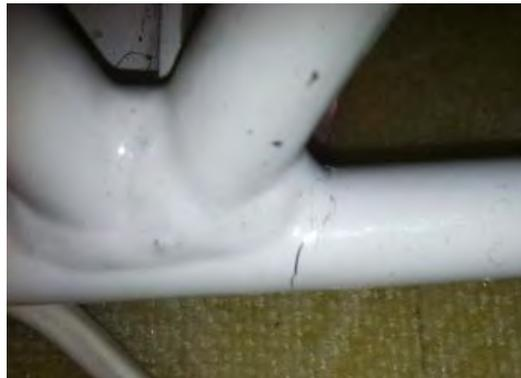
**Cracked rear tube at compression V tubes.**
