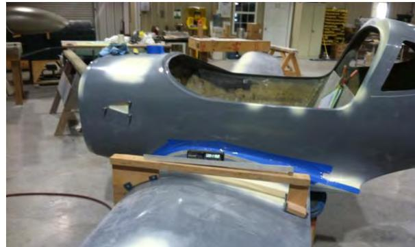
What the factory guys do is place the jig 18" out from the root. Set one wing based on the molded wing root. Once set we put a digital level on the top of the jig and get a measurement.
