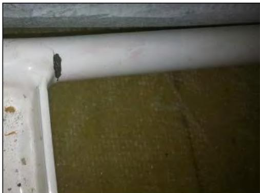
**Cracked forward tube at gear plate.**
