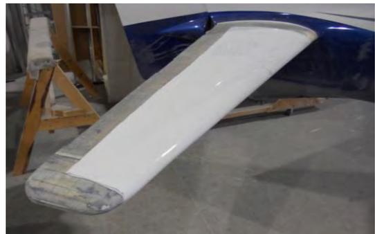
**Paint and gel coat are removed as shown to get a good base for the epoxy glue.**
