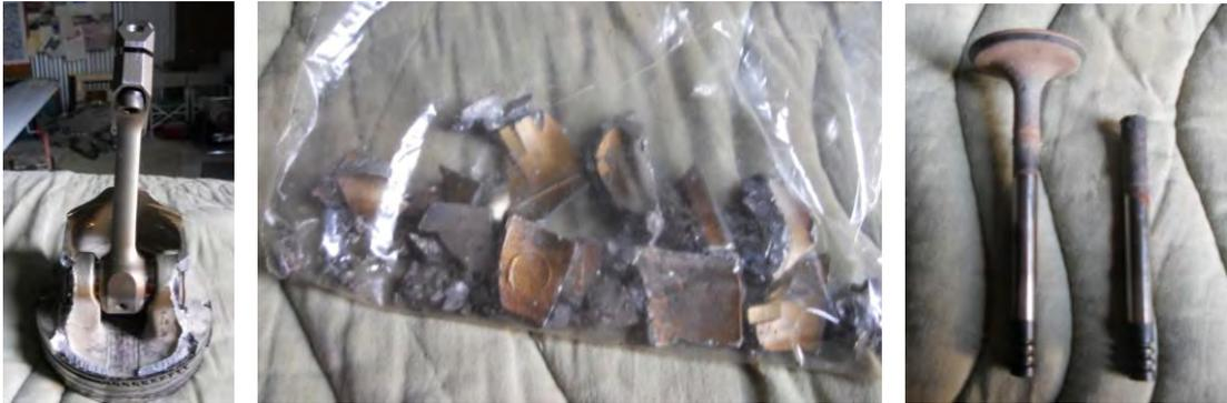
**Left: Piston photo showing broken skirt and bent rod.**
