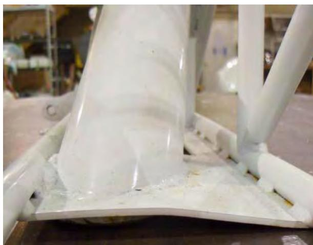
**Deformation of lower socket plate**
