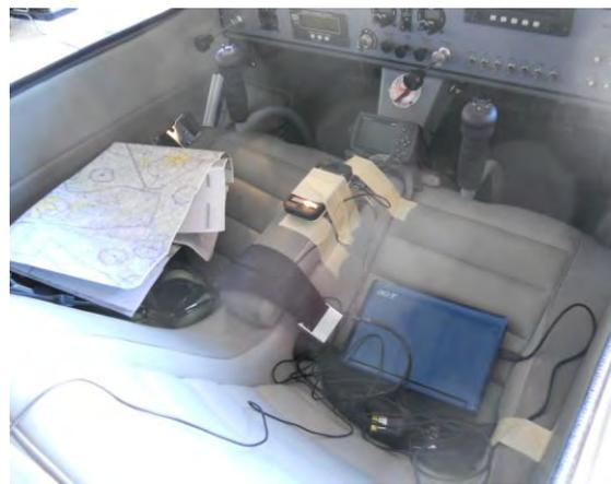
**Initial flights to record turbulence were made in my aircraft with a ViGYAN engineer in the right seat (left photo). Recent flights have been with just the very accurate accelerometer that measures forces in the pitch, roll, and yaw axis. This very small piece of equipment is also a self-contained Inertial Navigation System, a GPS, a magnetometer, and other capabilities. Everything is fed into a laptop computer that records all the data.**
