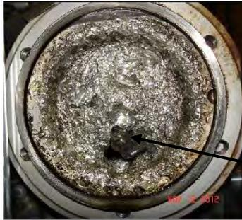
**Hole and valve head imbedded in piston.**
