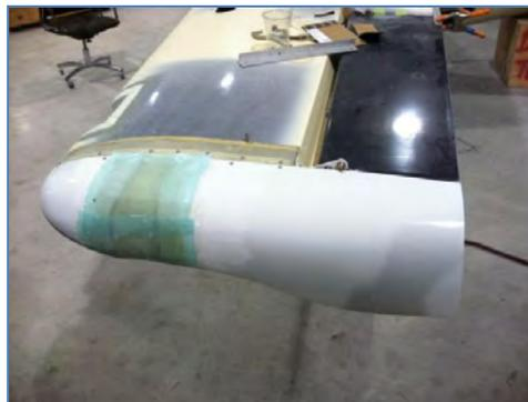
**The shortened “winglet” tips being fitted to the new 2013 EAB demo.**
