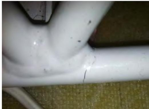
**Cracked rear tube at compression V tubes.**
