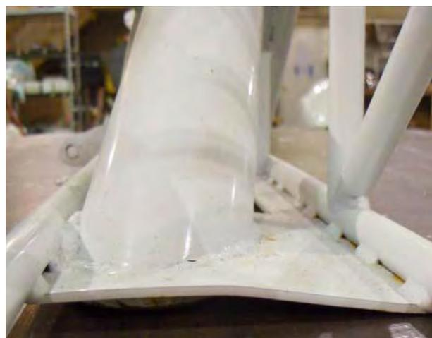
**Deformation of lower socket plate**
