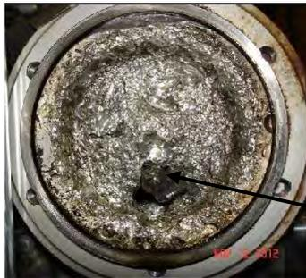
**Hole and valve head imbedded in piston.**
