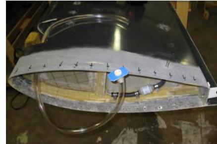
The left photo below shows yours truly sanding the outboard aileron hinge attach area where I added 6 plies of 8 oz. cloth. This is for reinforcing this area because I plan on extending the ailerons about 9" outward, or longer. The next photo I am sanding and adding the glass cloth.
