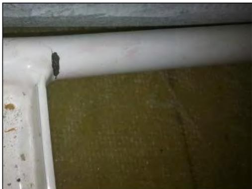
**Cracked forward tube at gear plate.**
