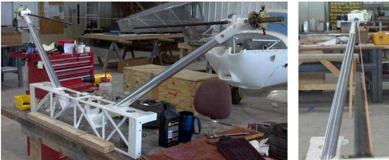
**Assembly on the bench ready to drill. Note the 1/2" steel tubes and tight drawn string.**
