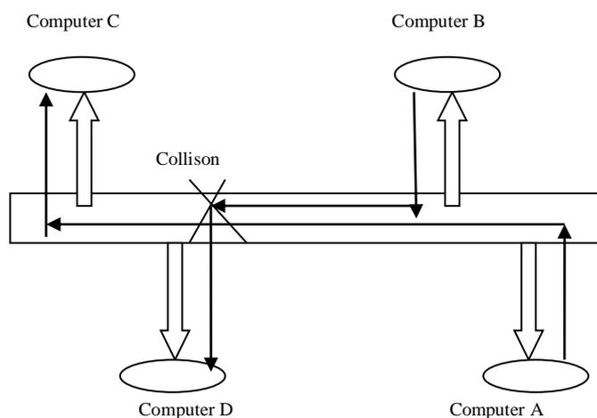
Fig. 1. Collision on Hub
