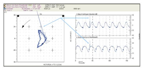
Figure 5 – Series of unfiltered orbit/timebase plots from bearing 6 showing random positive- and negative-going spikes due to electrostatic discharge.
