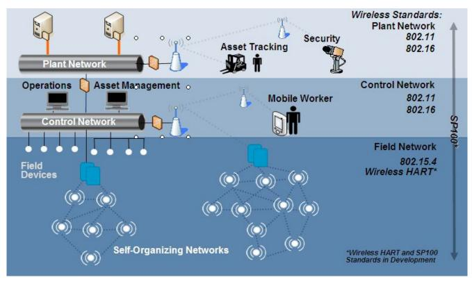
Currently, equipments available are Smart Wireless pressure and temperature transmitters, digital valve controllers, and vibration monitors along with a Smart Wireless Gateway to receive the transmissions and funnel the data to a control platform. Networks using self-organizing technology
