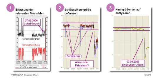
Fig. 2: Detecting critical changes in the process by evaluating available performance data
