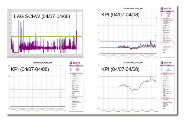
Fig. 4: Incipient crack of the shaft of a boiler feed pump  $\rightarrow$  increased bearing vibrations
