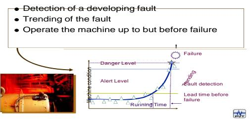
When an alert alarm occurs, there is lead time where the machine can still be operated with little or no performance degradation, and the development of the failure, its cause are determined and maintenance is planned ahead. Condition Monitoring permits monitoring of progressive failure modes in measurable terms, such as:
