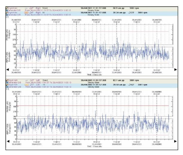
Figure 2 – Direct and 1X vibration trends on bearing 6 showing erratic behavior (top plot shows X probe, bottom plot shows Y probe).
