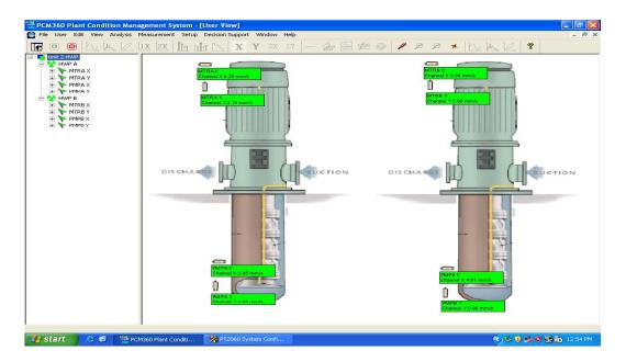
The decision to install the sensors at pump proved useful, and with the help of the diagnostic system installed the vibration spectrum plots indicated a 1 Hz component being the major source of vibration in the pumps, and further analysis was carried out
