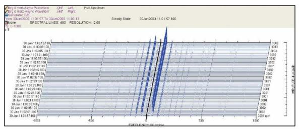
Figure 4 – Full-spectrum waterfall plot from bearing 6 showing predominantly 1X (50 Hz) vibration and small amount of 2X vibration (100 Hz), free from other harmonics or sub-harmonics.
