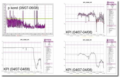
Fig. 3: Decline of process quality: condenser in off-design operation
