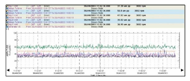
Figure 3 – Trend of overall vibration levels from Y probes on bearings 1-5 showing stable behavior.
