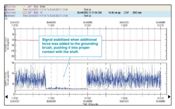
Figure 6 – Vibration trend showing effect of spring force on grounding brush.
