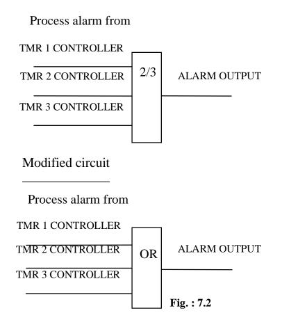
The RCA findings had revealed that the alarm was configured on majority voting philosophy of the TMR concept. But, due to its short-coming of not generating alarm in case of false signal simulation, or in case of single field element mal-operation it was decided to change the 2/3 logic into an OR GATE logic. This modification also had an additional benefit of taking a proactive action of replacing the faulty field element before the trip occurs.
