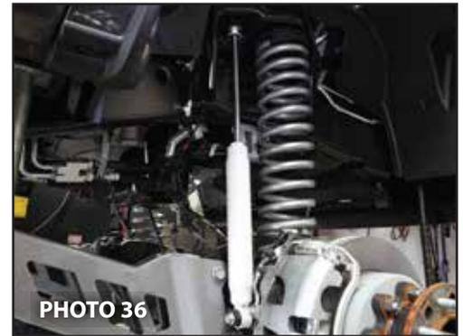
35. Install the shocks with the supplied new upper hardware and original lower hardware using a 21mm wrench for the upper nut and a 21mm socket and wrench for the lower hardware. (Photo 36)
