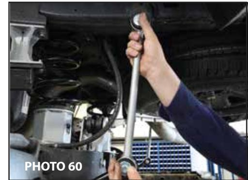
67. **IMPORTANT:** Double check all of the fasteners, bolts and components, making sure everything has been properly torqued as outlined in these instructions to factory specifications. This **MUST** be done prior to operating the vehicle. We recommend periodically checking all of the front suspension and lift kit components and fasteners to be certain they are tight and in proper working order.
