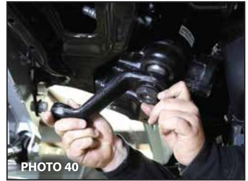
41. Loosen the drag link adjuster lock nuts. Turn the adjuster until the drag link is free.
