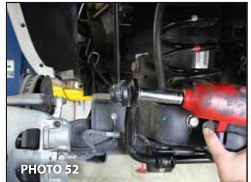
61. Open the existing hole in the factory lower track bar bracket with a 1/2" drill bit as shown. (Photo 55)
