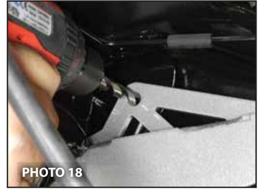
20. To mount the McGaughy's track bar relocation bracket, start by placing the factor bolt through the track bar bracket and drill the brace hole using a 7/16" drill bit. Place something firm between the crossmember and oil pan to prevent damage. **NOTE: The top hole on the bracket may or may not require drilling with a 1/2" drill bit, due to the production variances on Ram frames.** (Photos 17 & 18)
