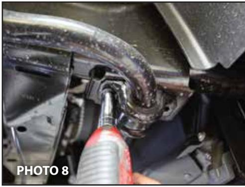
7. Remove the sway bar mounting bolts from the frame using a 15mm socket. (Photo 8)
