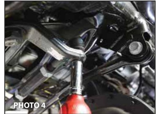
3. Remove the driver's side drag link to pitman arm nut using a 21mm socket. Use a tie-rod removal tool to avoid damaging you stock tie-rod ends. (Photo 4)
