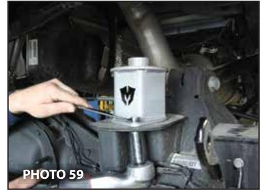
63. Place the McGaughy's 2-1/2" coil spring spacers on the axle and align with the existing holes. Mount the spacers using the provided 3/8" x 1 1/4" bolts, washers, and nuts. Re-install the coil springs.
