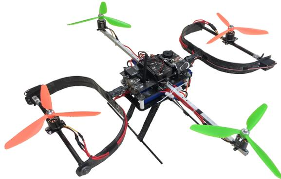
**Modelling and Attitude Stabilization of a Tilt-Quadrotor:**
