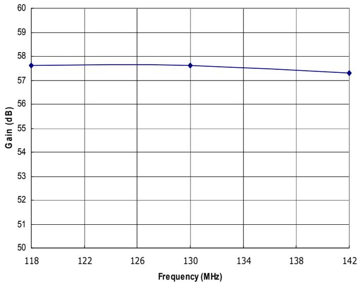
Figure 1: RFP118-142-350XR Typical gain @ P<sub>out</sub>=350W.
