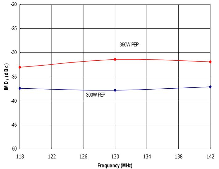
Figure 2: RFP118-142-350XR Typical IMD<sub>3</sub> @ 350W and 300W PEP, Δf=100kHz and Δf=10kHz.
