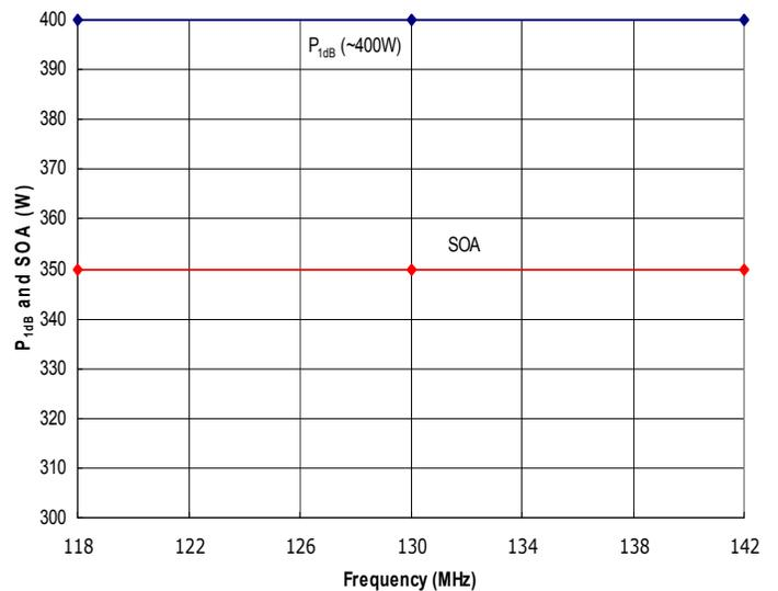
Figure 4: RFP118-142-350XR Typical P<sub>1dB</sub> and Safe Operating Area (SOA). The SOA assumes a 50 ohm load and adequate cooling of output transformers. Do not exceed the SOA shown above without first contacting RFMPT to discuss your application.
