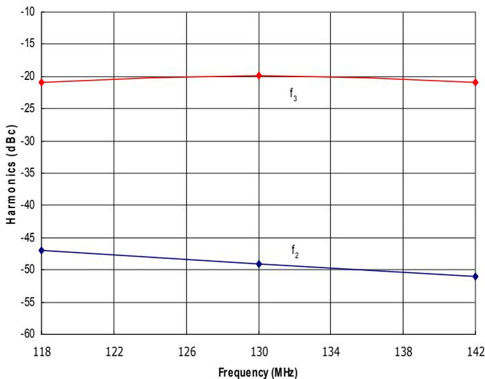
Figure 3: RFP118-142-350XR Typical f<sub>2</sub> and f<sub>3</sub> @ P<sub>out</sub>=350W.
