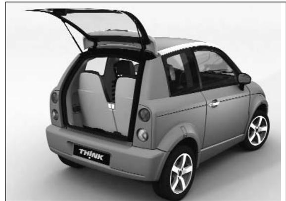
The 78th International Motor Show, held March 6-16 in Geneva, has a fine selection of electric cars and other alternate-power vehicles. Two notable exhibits are from Think: the City and the Ox. The two-seater City (above), redesigned at the end of 2007, is available with a choice of sodium or lithium-batteries, has a range of up to 180 km (112 miles) and a top speed of 100 km/hr (80 mph) from a 30 kW (peak) 3-phase motor.
