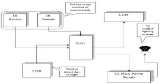
Fig.3: Block diagram of automatic light control system
