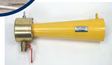
W 70 6" dia. Pneumatic Air Mover 3000 cfm output @ 90 psi
