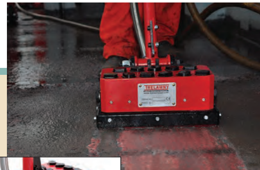
11 heads provide 33,000 BPM (11 x 3000 BPM)
