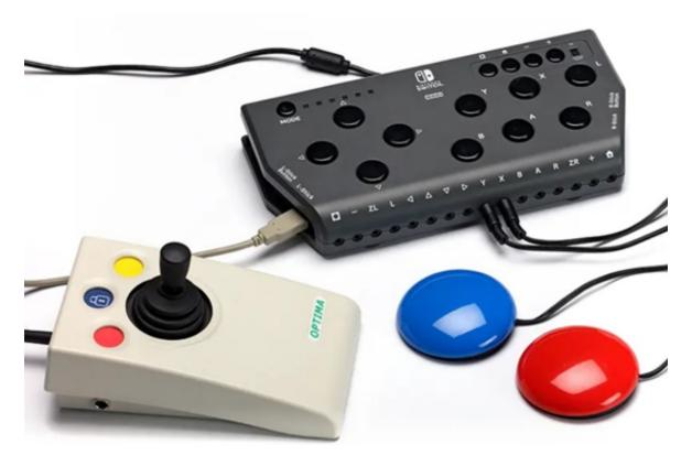
Picture shows joystick and two switches connected to the gaming cable dock
