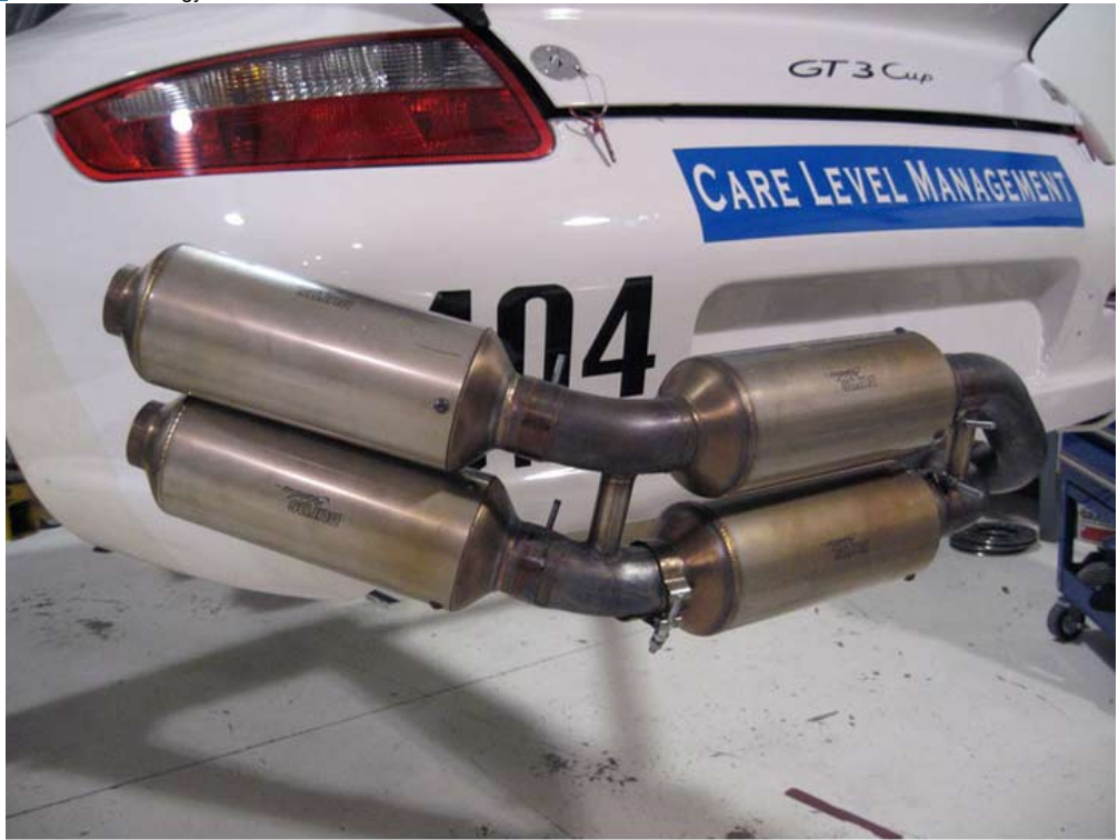
Figure 2 - Wild muffler configuration developed by Competition Motorsports for Laguna Seca. It is about the only way to get a GT3 Cup car to pass.
