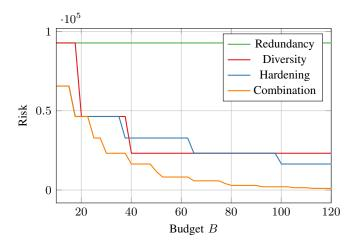
Fig. 3. Security risk in the water-distribution network when investing only in redundancy, only in diversity, only in hardening, or in their combination.
