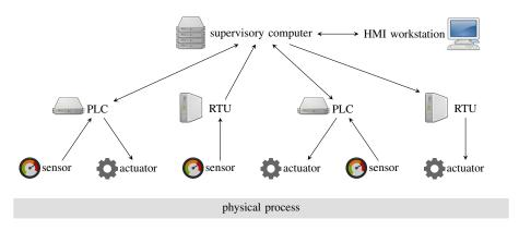
Fig. 1. Example cyber-physical system. Arrows represent flows of sensor data and control signals.
