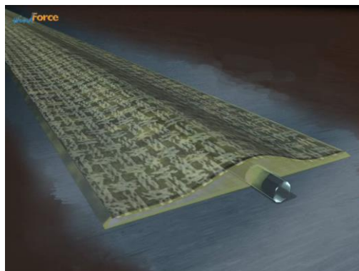
Figure 5: Fibre Optic Sensor bonded to steel surface and covered with protective tape and epoxy
