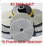
lars each. The grit sizes in each set are (2) #50, (1 each) #100, #200, #400, #800, #1500, #3000, and #6000. Plus a hook and loop-backing pad drive disk. The drive pad has a standard 5/8-11 thread.
