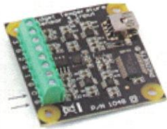
Insert bean temperature probe wires into the G and 0 terminals.
