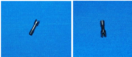
Fig 7- a,b-Retrieved internal hex with prepared notches
