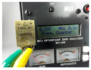
6. Analyzer\* output measured for a 10 MHz crystal
