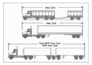
Figure 4: Length of Combination of Vehicles
