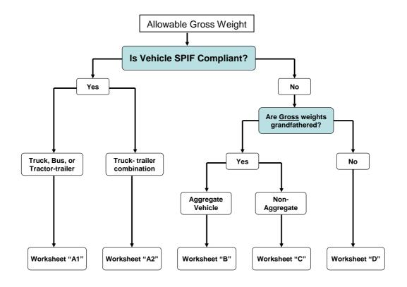
An 'aggregate vehicle' means a vehicle or vehicle combination that is designed for dumping or spreading of sand, gravel, crushed or uncut rock, asphalt, slag rubble, or any mixture thereof and that is transporting a load consisting mostly of any of these materials – Reg 413/05 s2 (Road salt is not considered to be an aggregate product.)
