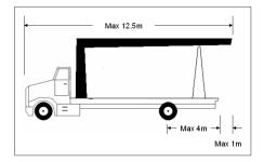
Figure 6: Overhanging Boom of a Rear-Facing Crane
