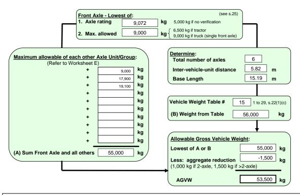
The truck in this configuration is equipped with a rigid lift axle which disqualifies the combination from being SPIF.
