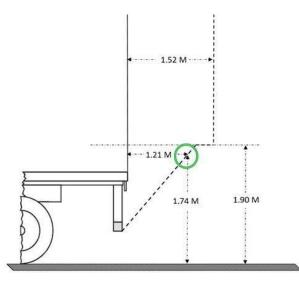
Figure 1: Dimensional Limits for Aerodynamic Devices on Rear of Vehicle
