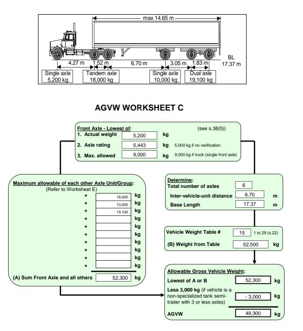
The triaxle semi-trailer in this example is a bulk tanker equipped with a rigid lift-axle and a non-load-equalizing suspension – either of which disqualifies the combination from being SPIF.
