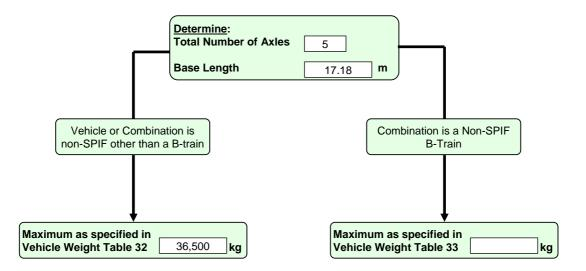
The non-dump semi-trailer in this example is equipped with a rigid air-lift axle which disqualifies the combination from being SPIF. Other than dumps or tankers, all grandfathering protection for non-SPIF semi-trailers with 3 or less axles has expired.
