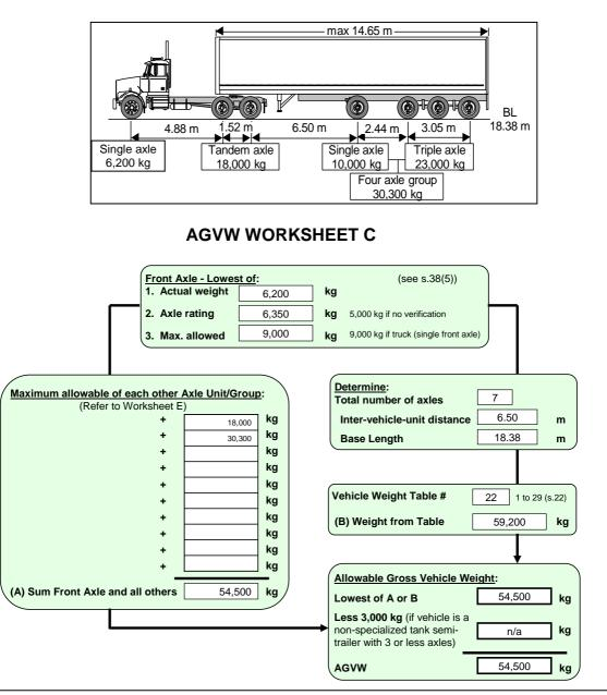
The non-dump semi-trailer in this example is equipped with a rigid lift-axle and a non-load-equalizing suspension – either of which disqualifies the combination from being SPIF.
