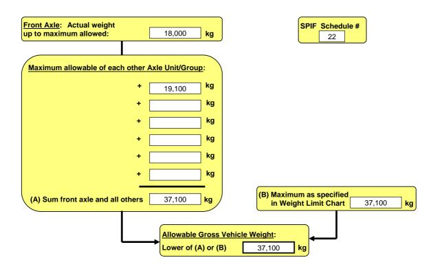
The wheelbase of this truck is 6.0m (measured from centre of tandem to centre of tandem), which allows the maximum AGVW. If the wheelbase is less than 6.0m, the AGVW is limited to 32,000 kg, Reg 413/05 schedule 22.
