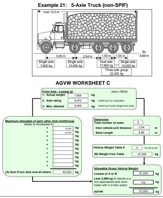
The 5-axle truck in this example is equipped with a rigid lift-axle, which disqualifies it from being SPIF. If, as illustrated, this is a log truck, during Freeze-Up the AGVW would be: 37,200 kg + 10% = 40,920 kg, HTA s119.
