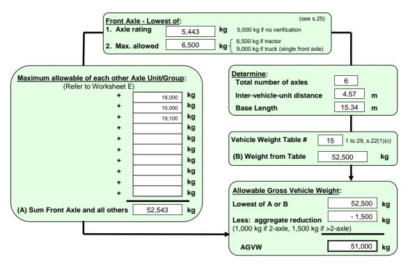
The end-dump semi-trailer in this example is equipped with a rigid lift-axle and a non-loadequalizing suspension – either of which disqualifies the combination from being SPIF.
