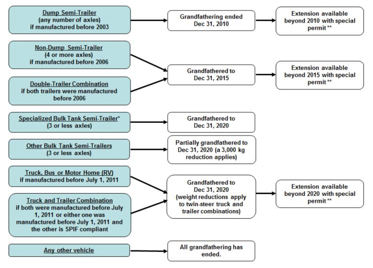
\* Specialized tankers include a carbon dioxide tank semi-trailer, cryogenic tank semi-trailer or tag-axle tank semi-trailer.
