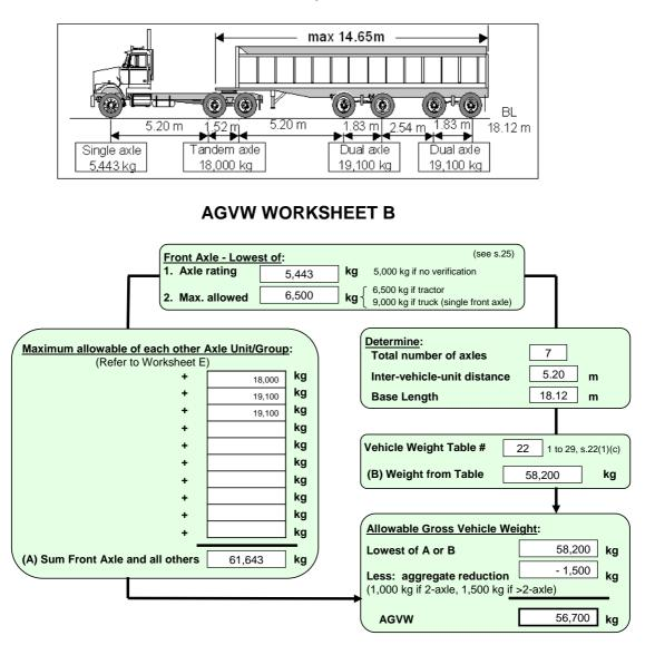
The dump semi-trailer in this example is equipped with rigid lift-axles, which disqualify the combination from being SPIF.
