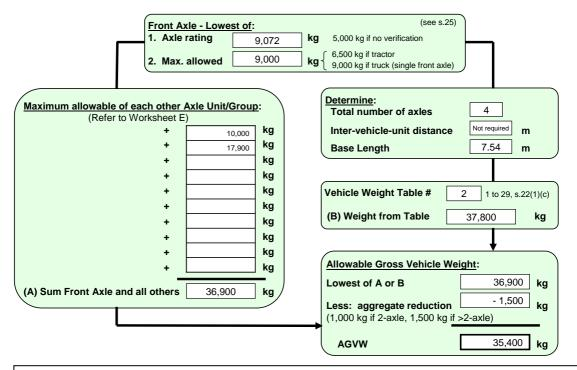
The truck in this example is equipped with a rigid lift axle which disqualifies the truck from being SPIF. Aggregate vehicle means a vehicle that is designed for dumping or spreading aggregate product and is loaded with aggregate product. Aggregate product includes sand, gravel, crushed or uncut rock, asphalt, slag, rubble, or any mixture thereof – but does not include salt, Reg 413/05 s2.
