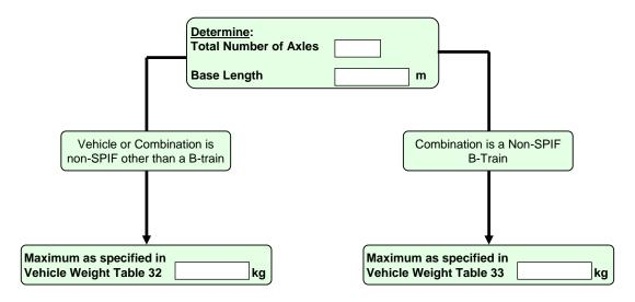
This worksheet is used for any non-SPIF vehicle or combination of vehicles where:
