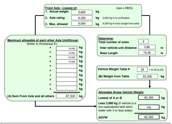
The semi-trailer in this example is equipped with rigid lift-axles on non-load-equalizing suspensions, either of which disqualifies the combination from being SPIF.
